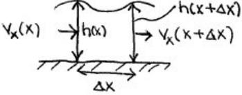
$$\Rightarrow \frac{\partial h}{\partial t} + \frac{\partial}{\partial x} \left( \int_0^h v_x dy \right) = \frac{\partial h}{\partial t} + \frac{\partial Q}{\partial x} = 0 \quad (6.16c)$$
