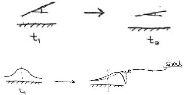
$\therefore$  In the case of slow-drying paint, when there is a bump, Eq. (6.16d) dictates that the bump grows! However it never forms a shock because in reality, one has to consider effects of surface tension.
