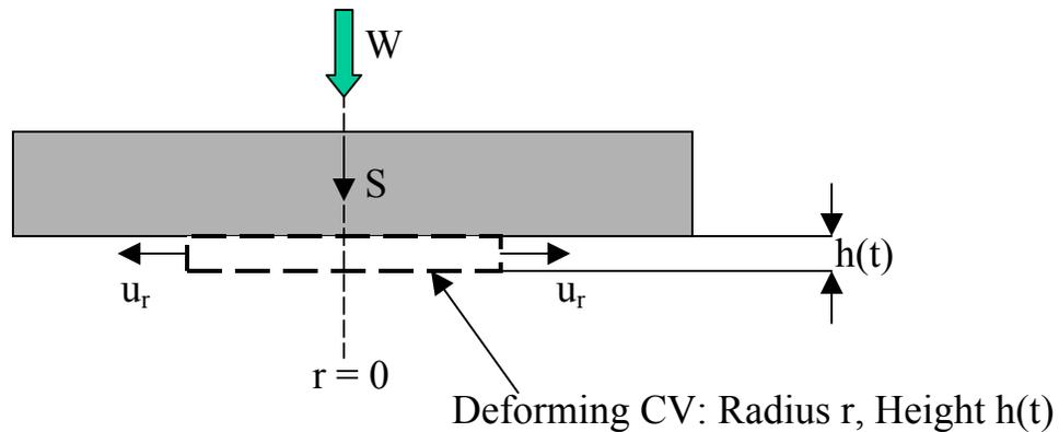
$$0 = \frac{d}{dt} \int_{CV} \rho dV + \int_{CS} \rho (\vec{V} - \vec{V}_{CS}) \cdot \vec{n} dA$$
