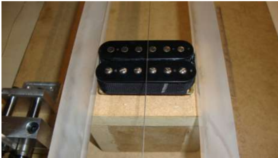
Figure 7.6 – Humbucker used to output frequency signal to amplifier.
