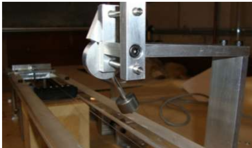
Figure 7.5 – Mechanical pendulum device used to impulse string.
