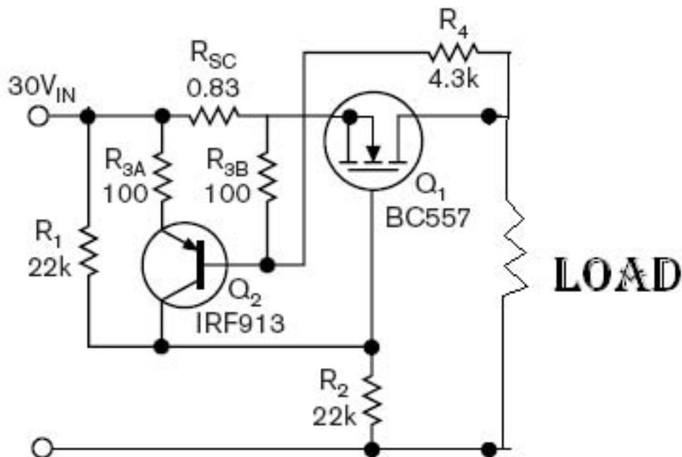
**Figure 1** This circuit adds foldback current limiting to a linear regulator.
