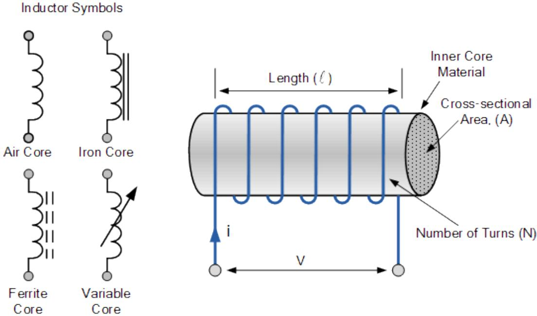
Inductor is an electrical component storing an electrical energy in form of a magnetic field  $\vec{B}$ . When current  $i$  flows to the inductor, the magnetic field forms within the magnetic core surrounded by a conducting coil carrying  $i$ . If  $i(t)$  is time-varying, then  $\vec{B}(t)$  is also time-varying. Then Faraday's law of induction is applied; The equation of Faraday's law of induction for a closed loop is
