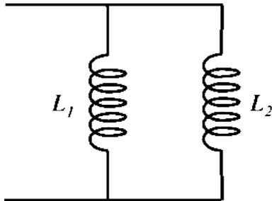
$$\begin{aligned} \tilde{Z}_{eq} &= \left( \frac{1}{j\omega L_1} + \frac{1}{j\omega L_2} \right)^{-1} = \left( \frac{j\omega L_1 + j\omega L_2}{-\omega^2 L_1 L_2} \right)^{-1} = -\frac{\omega L_1 L_2}{jL_1 + jL_2} = j\omega \frac{L_1 L_2}{L_1 + L_2} = j\omega L_{eq} \rightarrow L_{eq} \\ &= \frac{L_1 L_2}{L_1 + L_2}. \end{aligned}$$
