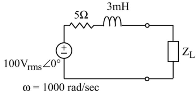
a) Determine the load impedance  $Z_L$  that absorbs the maximum average power from the source.
