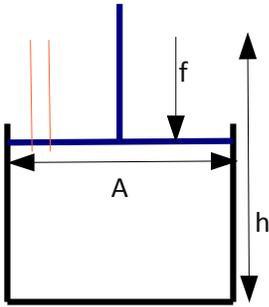
A force  $f$  applies on the piston, since the area of the piston (and of the base of the cylinder also) is  $A$ , the pressure imposed by the piston on the fluid will be  $f/A$ .
