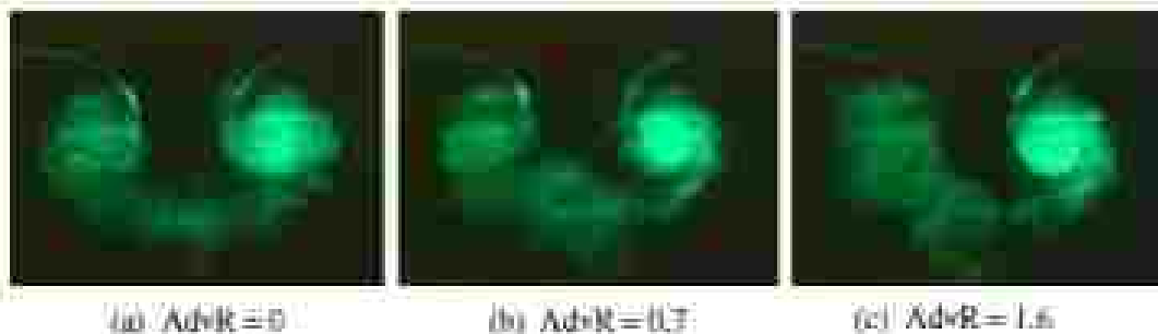
Figure 2.3: The trailing vortex pair at various spin rates at Reynolds number of 5.67 \times 10^4 . Spin causes an asymmetric vortex wake (Taken from Potts, 2005).
