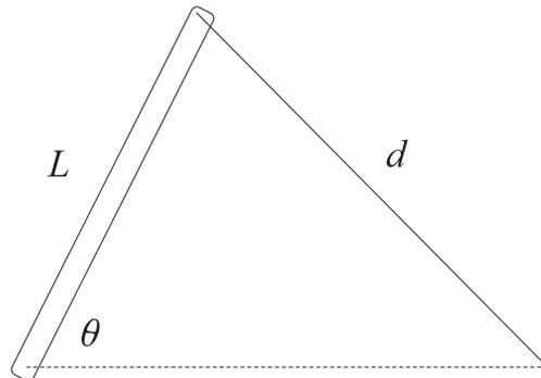
**Problem 18.57** The slender bar weighs 40 N and the crate weighs 80 N. At the instant shown, the velocity of the crate is zero and it has an acceleration of  $14 \text{ m/s}^2$  toward the left. The coefficient of kinetic friction between the horizontal surface and the crate is  $\mu_k = 0.2$ . Determine the couple  $M$  and the tension in the rope.
