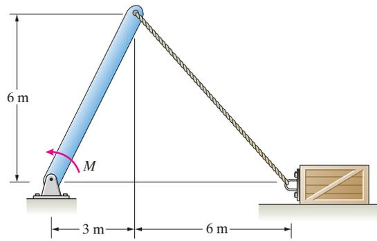
**Solution:** There are six unknowns ( $M, T, N, O_x, O_y, \alpha$ ), five dynamic equations, and one constraint equation. We use the following subset of the dynamic equations.
