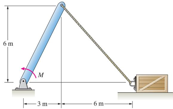
**Solution:** There are seven unknowns ( $M, T, N, O_x, O_y, \alpha, f$ ), five dynamic equations, one constraint equation, and one friction equation. We use the following subset of the dynamic equations.
