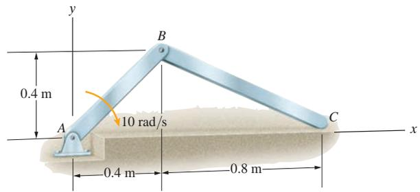
**Solution:** We first perform a kinematic analysis to find the angular acceleration of bar  $BC$  and the acceleration of the center of mass of bar  $BC$ . First the velocity analysis:
