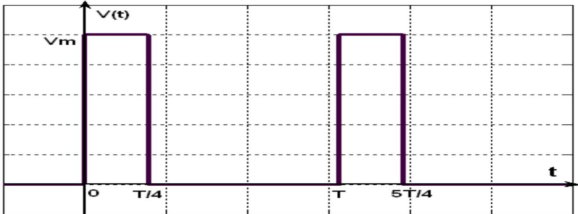
$$T=20[\text{msec}], V_m=100[\text{v}], \omega_0=2\pi/T =100\pi [\text{rad/sec}]$$
