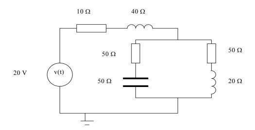
Q3. In the following circuit calculate the voltage across Z. What current is flowing in the circuit? What energy is stored in the circuit? The supply frequency is 100 rad/s.
