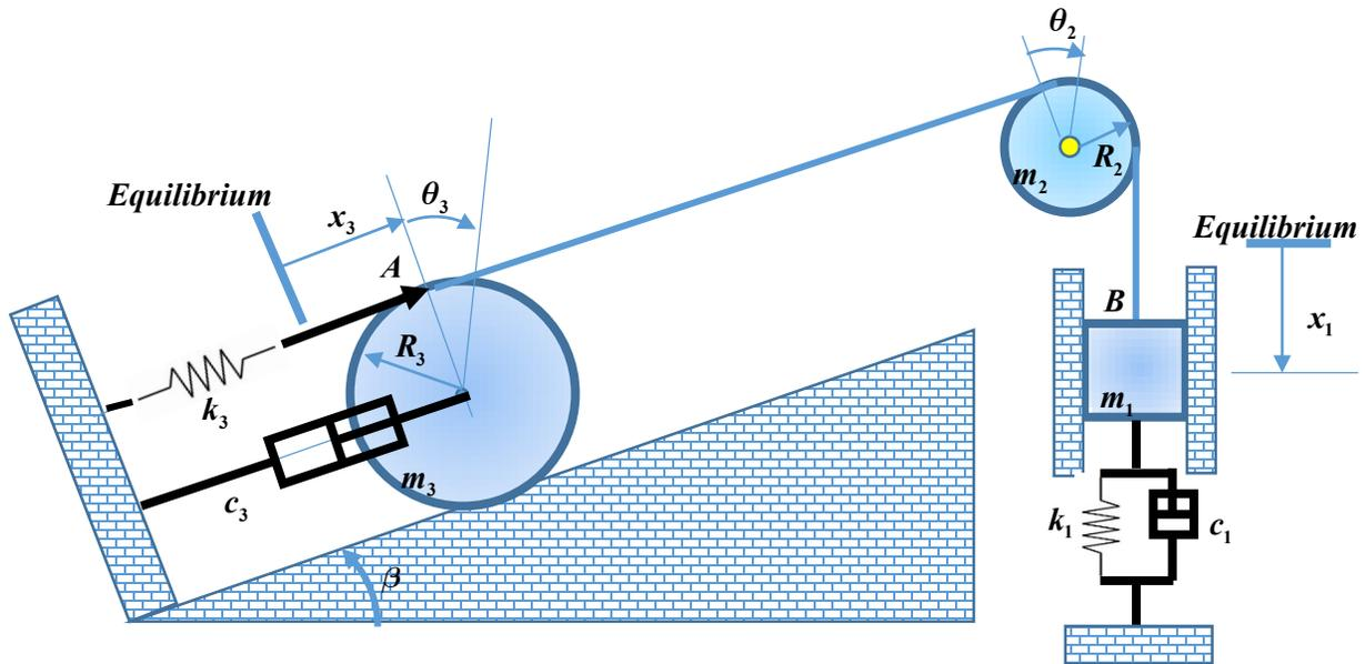
$$\left( m_1 + \frac{m_2}{2} + \left( \frac{3}{8} \right) m_3 \right) \ddot{x} + \left( c_1 + \frac{c_3}{4} \right) \dot{x} + (k_1 + k_3)x = 0$$
