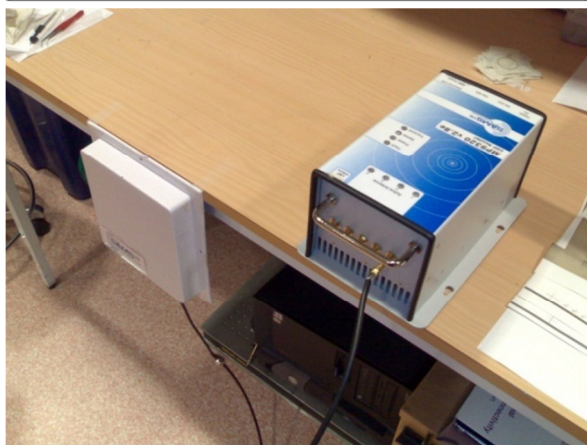
Figure 1. Stationary RFID reader (lower) controlled by a specially developed software to sweep output power and retrieving backscattered signal strength (RSSI).
