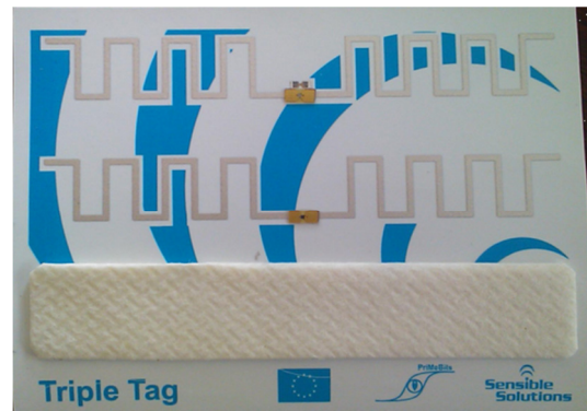
Figure 5. Example of triple tag, with reference tag in the middle and one sensor equipped tag above and one below
