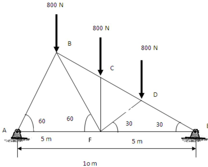
a) Analysis framework shown above by using method of joints .Make sure that you are carefully identify whether individual elements are in tensions or compression.
