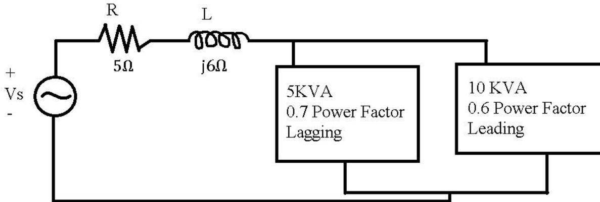
Load 1 is the 5 KVA load and Load 2 is the 10 KVA load. Loads 1 and 2 are operating at their rated voltages of 220 V rms.
