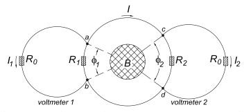
Two identical voltmeters with internal resistance  $R_0 \gg R_1, R_2$  probe the central circuit, the first connecting to points a and b, and the second connecting to points c and d. The positive leads of the voltmeters are attached to points a and c, which defines the sense of currents  $I_1$  and  $I_2$  to be as shown. We suppose that no magnetic flux from the solenoid passes through outer loops 1 and 2.
