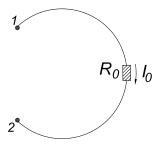
Discuss the relation of the meter reading to the difference  $V_1 - V_2$  in the scalar potential V between points 1 and 2, and to the line integral  $\int_1^2 \mathbf{E} \cdot d\mathbf{l}$  along the circuit being probed, in the absence of the voltmeter.
