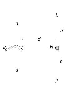
To predict the behavior of the voltmeter, I used the NEC4 simulation [22] with the LD command to generate a resistance  $R_0$  of 1 megohm. Results are given in Table 1 for a drive voltage  $V_0 = 1$  volt.
