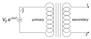
The role of the 1:1 transformer is to present a voltage drop between terminals 1 and 2 equal to the voltage drop  $V_0 e^{-i\omega t}$  of the power source. This voltage drop is equal, to a good approximation to the difference in the electric scalar potential between terminals 1 and 2 (as well as that at the terminals of the power source).
