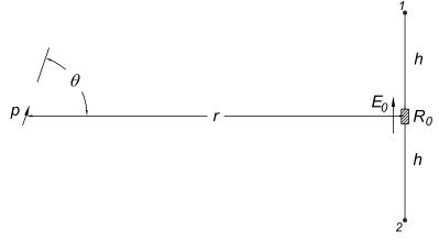
The voltmeter is in effect a dipole receiving antenna with a high resistance between its terminals. The  $\mathcal{EMF}$  across the terminals will be essentially the same as if the resistance  $R_0$  were infinite, *i.e.*, the open-circuit voltage. This voltage has been discussed elsewhere [20], and the simple result is that
