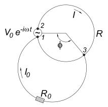
The two loops in the resulting configuration have self inductances  $L_0$  and L, and mutual inductance  $M \approx L\phi/2\pi$  since the flux through meter loop due to current I in the single-turn inductor is largely due to the current on the segment 1-3, which segment is associated with self inductance  $L_{13} \approx L\phi/2\pi \approx M$ .
